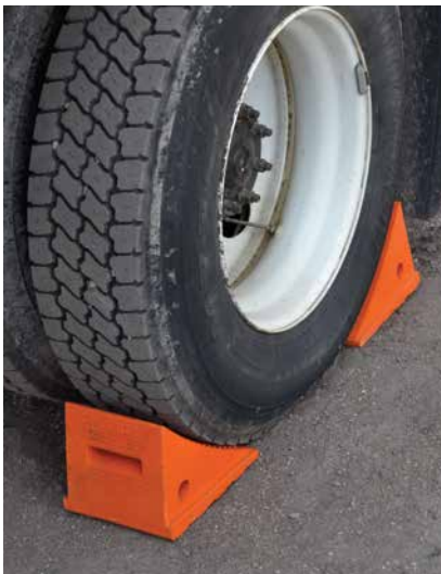
Monster urethane chocks model UC1500 used on a utility truck
